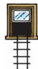
ESCAPE LADDER. Folding ladder that is stored under a window.
